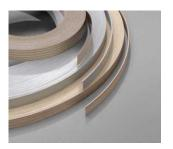
EGGER ABS edging tape is a thermoplastic edging product with protective and decorative properties for finishing the narrow sides of wood-based panels. EGGER ABS edging is made of ABS and is uniformly coloured through. A universal bonding agent (primer) is applied to the reverse side as standard.
