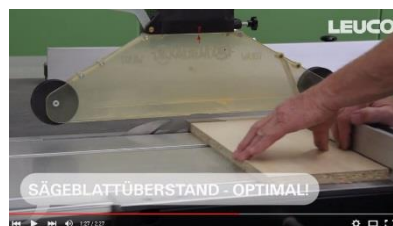
(to adjust saw blade projection optimally)
